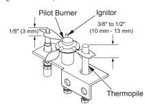
Figure 18 - Correct Pilot Flame Pattern - Millivolt Assembly
